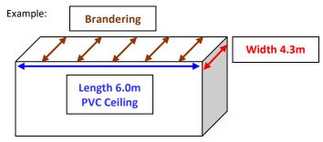
If the length of the room is 6.0m and the width of the room is 4.3m you will calculate as follows:  $4.3m \div 0.25 = 18$  panels. The specifications are thus 18 panels x 6.0m
