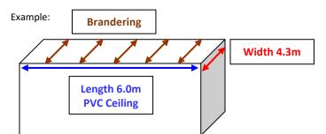
If the length of the room is 6.0m and the width of the room is 4.3m you will calculate as follows:  $4.3m \div 0.30 = 15$  panels. The specifications are thus 15 panels x 6.0m
