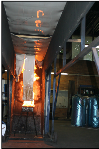
Figure 4.2.1: Front portion of ceiling dropped out after 5 minutes
