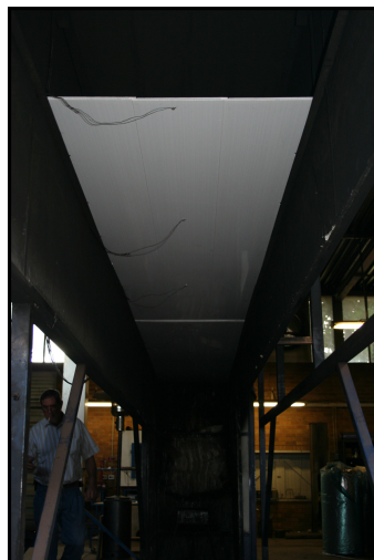
Figure 3.3.2: Test installation prior to ignition of fire source
